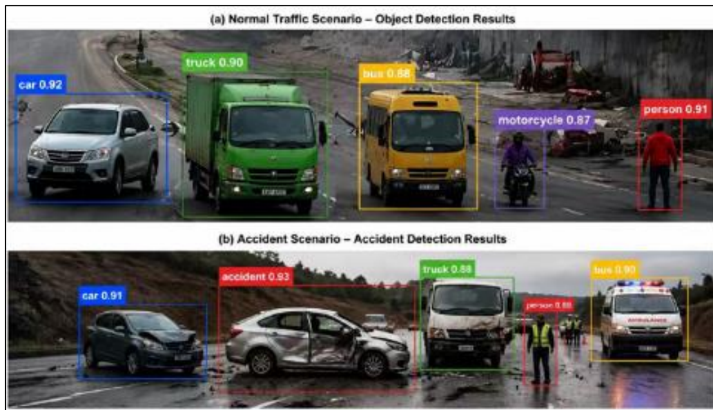
Figure 4 Qualitative detection results of the proposed YOLOv8 framework under normal and accident traffic scenarios.
